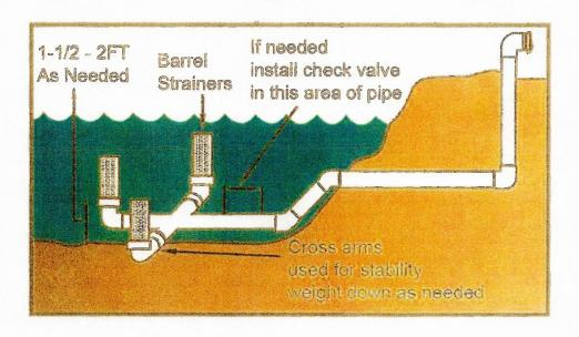
Cross arms must be supported by a substantial foundation block or blocks, approved by Wilton Fire.
