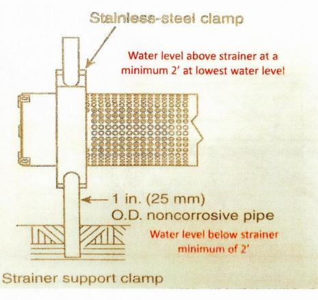
Strainer support clamp must be attached to a substantial foundation block, approved by Wilton Fire.
